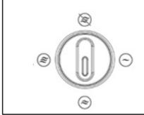
**3.** Turn the switch to " ", it means the heater is working and on the maximum heating position (2500W).
