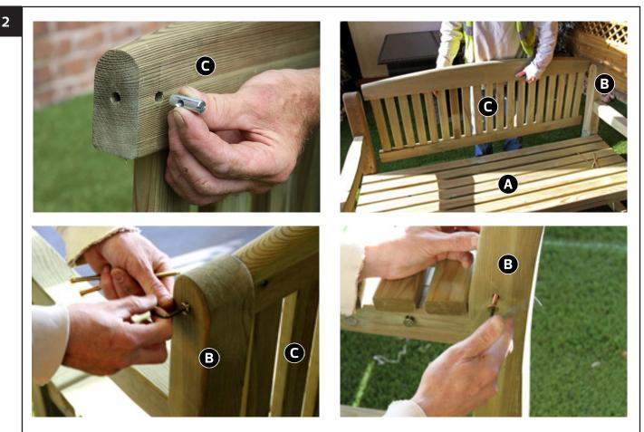
Insert 4 Cross Dowels into 10 mm holes to rear of Back Assembly (C) ensuring slots face outwards (as shown, which allows for aligning dowels with bolts using a slot head screwdriver). Position the Back Assembly between side assemblies and insert 2 bolts per side and carefully thread bolts into cross dowels.
