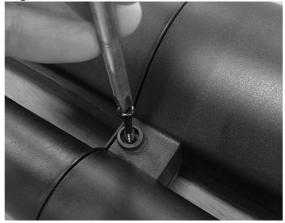
Insert both tubes into the main body and screw together with a large tube screw.
