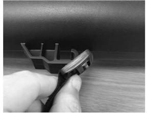
Hook the rear securing clasp of the collection bag onto the main body hook.
