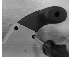
To assist with the handle fitting flush with the main housing, it may be necessary to loosen the two casing screws, by 2 complete turns and apply downward pressure on the front handle to insert. Tighten the two screws when housed.
