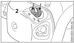
► Depress the outer ring (arrows) of the choke knob (2) and then turn it to <u>I</u>.
