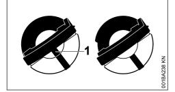
Left: Bottom of cap is twisted – inner mark (1) in line with outer mark. Right: Bottom of cap in correct position – inner mark is under the grip. It is not in line with the outer mark.
