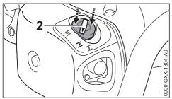
► Depress the outer ring (arrows) of the choke knob (2) and then turn it to ∠. Also use this setting if the engine has been running but is still cold.
