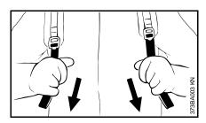
Pull the straps downwards to tighten the harness
