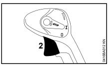
• Operate the throttle trigger (2).
