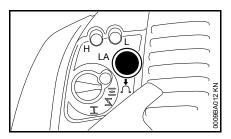
Press the fuel pump bulb at least eight times – even if the bulb is filled with fuel.
