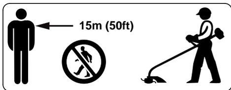
There is a risk of accident from ejected objects within a wide area around the working space, so you must ensure that there is no-one within a 15 m radius of the machine. This distance must
