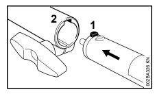
Push the lug (1) on the drive tube into the slot (2) in the coupling sleeve as far as stop.
