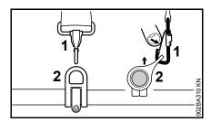
Press down the bar on the carabiner (1) and pull the carrying ring (2) out of the carabiner.
