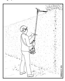
Hold the hedge trimmer vertically and swing it in an arc to make maximum use of its reach.
