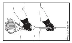
Right hand on control handle, left hand on handle hose on drive tube, even if you are left-handed. Wrap fingers and thumbs firmly around the handles.
