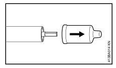
Pull the protective cap off the end of the drive tube and keep it in a safe place.
