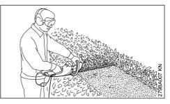
If the hedge is wide, cut it in several passes – one hand on the front switch lever – one hand on the control handle.
