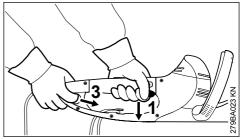
Release the trigger switch (1) and auxiliary switch (3).
