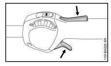
Depress throttle trigger lockout and pull the throttle trigger – the choke knob moves to the Run I position.
