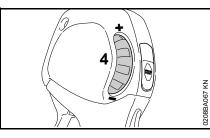
The throttle set wheel (4) enables the travel of the throttle trigger to be preset anywhere between idle and full throttle.
