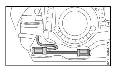
• Check the pickup bodies in the fuel tank annually and have them replaced when necessary
