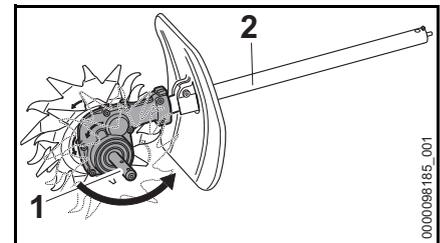
the axle (1) must be located below the shaft (2). The arrows on the gear unit indicate the direction of rotation
