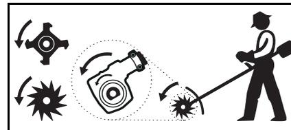
Arrows on the blades show the direction of rotation. The arrows on the rotor blades must point in the same direction as the arrows on the gear.
