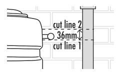
When used with a diverter, rainwater is diverted into the butt until it is full. Once full, excess water will continue down the pipe and into the drain.
