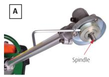
With the unit tipped up remove the shaft nut from the spindle and lock the gearbox with allen key.
