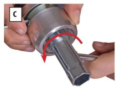
Keeping the shaft locked tighten with tube spanner supplied - remember left hand thread!
