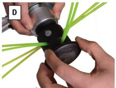
Screw on the plastic line hub, left hand thread!
