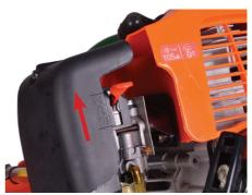
Move the red lever up to set the choke to enable easier starting especially in cold weather. Once engine is running move lever into the run position.
