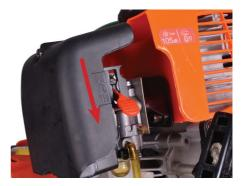
Adjust the handle for comfort and for use on sloping ground
