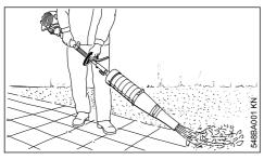
Always hold the unit firmly with both hands on the handles. Right hand on control handle, left hand on loop handle on the shaft, even if you are left-handed. Wrap your fingers and thumbs around the handles.
