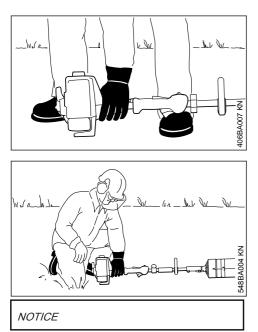
Start your machine on a clean surface only to ensure that no dust is sucked in.
