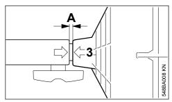
When correctly mounted, the intake screen (3) must be flush with the coupling sleeve (gap 'A' no more than 5 mm).
