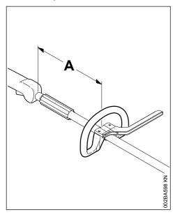
By changing the distance (A), the handle can be moved into the best position for the operator and application.
