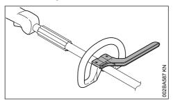
The barrier bar comes as a standard with the machine and must be mounted to the loop handle.
