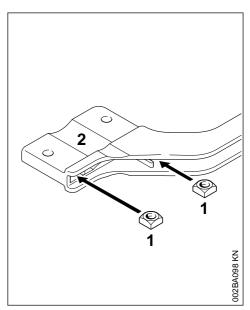
► Insert the square nuts (1) in the barrier bar (2) - the holes must line up
