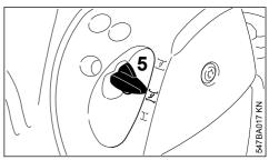
► Press in the choke lever (5) and turn it to <u>∠</u> at the same time.
