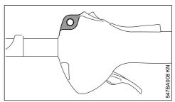
The carrying ring is integrated in the front end of the control handle.
