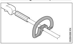
The new machine is delivered with the loop handle pre-assembled on the unit.
