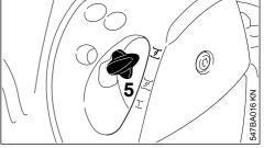
► Press in the choke lever (5) and turn it to <u>I</u> at the same time.
