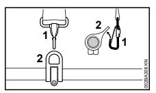
Attach the carabiner (1) to the carrying ring (2) on the drive tube – hold the carrying ring steady.
