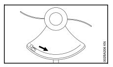
An arrow on the deflector (inside and outside) shows the correct direction of rotation of the cutting attachments.
