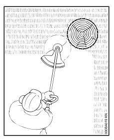
Nylon line achieves a soft cut for edging and trimming around fence posts, trees, etc. – less risk of damaging tree bark.
