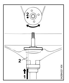
To block the shaft, insert a suitable tool (1) through the holes (2) in the deflector and thrust plate – turn the thrust plate back and forth if necessary
