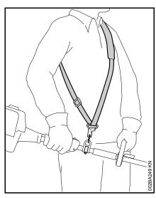
• With the engine running, attach the machine to the shoulder strap.
