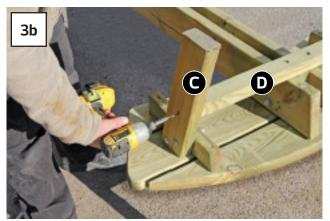
Position Leg Brace (D) on to Seat Bars (as shown in fig 3a), and fix in position using Two 80mm screws. Attach Legs to Leg Brace with two 80mm screws. See Fig 3b. Repeat for remaining Leg Braces.
