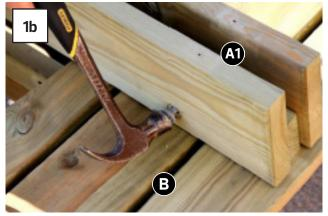
Position Seat Bars (A1) onto two. Seat Assemblies (B) as shown in Fig 1a, align bolt holes and insert 130mm bolts (Fig 1b). Attach 30mm washers, spring washers and nuts. Do not fully tighten at this stage. Repeat process using Seat Bars A2 and remaining Seat Assemblies.
