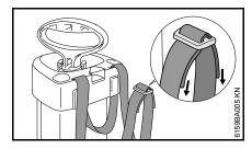
Thread the ends of the strap through the buckle.
