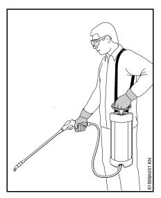
Put the strap over your left shoulder so that the unit hangs at your side. To ensure the unit can be quickly thrown off in an emergency, do not wear the strap across your chest.
