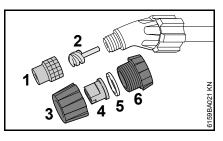
Unscrew the hollow cone nozzle (1) with spinner insert (2) from the wand
