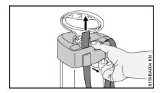
Ease the housing outwards and thread the strap through the openings from below.
