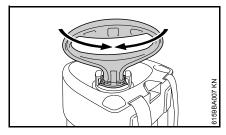
Rotate the pump handle about a quarter turn until it disengages and can be moved up and down freely.
