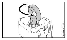
Push the pump handle downwards and turn it until it engages.
