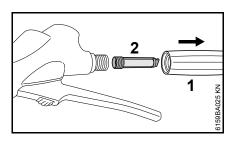
Unscrew the handle (1) from the spray gun and take out the filter (2).
