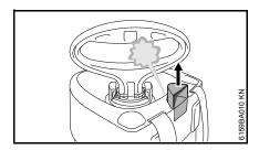
Pull the piston manometer up all the way – pressure is released – wait until tank is completely depressurized.
