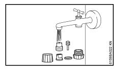
Rinse out all parts under running water and then reassemble.
