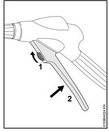
Push locking lever (1) upwards – the trigger (2) is unlocked and can be operated.
