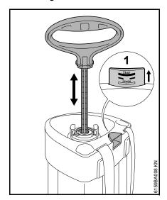
Move the pump handle up and down several times – the pressure in the solution tank rises.
