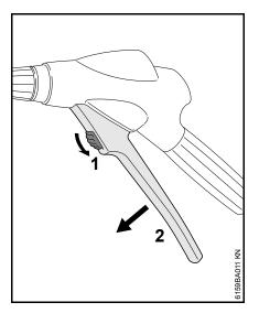
Push the locking lever (1) downwards – the trigger (2) is locked to reduce the risk of accidental operation.
