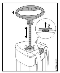
Pressurize the tank – move the unlocked pump handle (1) up and down several times until piston manometer (2) shows a pressure of 2 bar (29 PSI).
