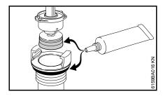
Lubricate the piston cup seal and Oring with a food-safe grease.
