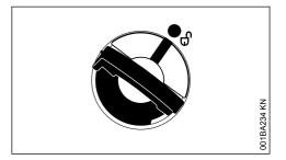
Marks on tank cap and fuel tank must line up.
