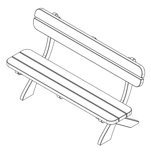
$(W \times D \times H) 1.60 \text{m} \times 0.62 \text{m} \times 0.88 \text{m}$
