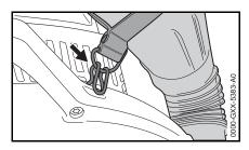
Attach D-ring to the hook on the blower housing.
