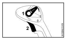
The throttle trigger (2) can be locked in any position.
