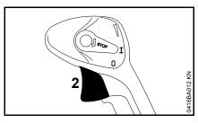
Blip the throttle trigger (2) – the choke knob automatically returns to T Turn the choke knob to I.
