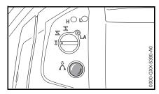
Press the fuel pump bulb at least 6 times – even if the bulb is already filled with fuel.
