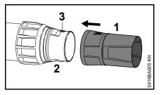
Push the nozzle (1) onto the blower tube (2) and engage it on the lugs (3).
