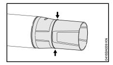
The front end of the nozzle wears away due to abrasive ground contact during operation. The nozzle is subject to normal wear and tear and must be replaced when the wear mark is reached.
