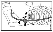
• Engage the throttle cable (4) with sleeve (5) in the retainer (6).
