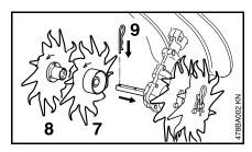
rotate the inner right-hand rotor blade (7) on the shaft until it can be pushed into position – check the direction of rotation again - arrows -
