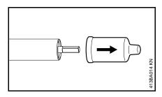
Pull the protective caps off the ends of the shaft and keep them in a safe place for later use – see "Storing the Machine"
