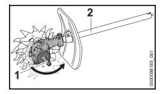
the axle (1) must be located below the shaft (2). The arrows on the gear unit indicate the direction of rotation
