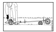
Place the machine on the ground: It must rest securely on the machine support. Rest the deflector end of the drive tube on a raised support (e.g. mound, log, brick).
