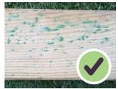
Most Zest products are pressure treated which protects the timber from rot for many years. Pressure treatment can result in a small amount of 'green spotting' on the surface of new timber caused by natural salts leaving the wood. This will fade away over time.
